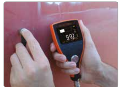
Ideal for measuring the material thickness of coated materials, ignoring the paint thickness (EE mode).
