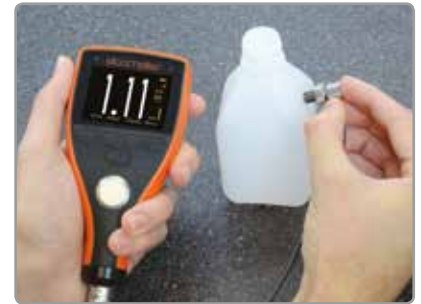
Ideal for measuring the material thickness of thinner materials such as plastics.
